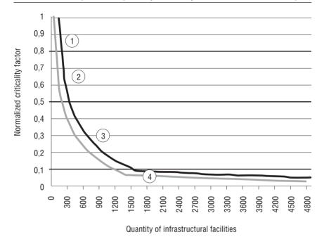
Fig. 3.3.3. Example of infrastructural facilities ranking based on their «criticality» level
